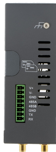
Figure 10. SIM Slot, Earth point, Terminal block
