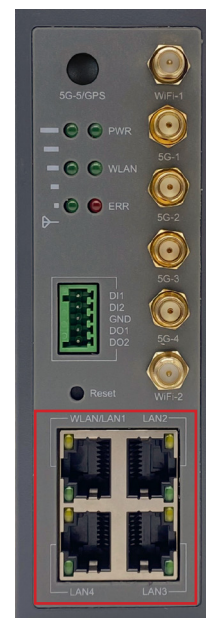
Figure 14. LAN/WAN Connectors (non-GPS version)
