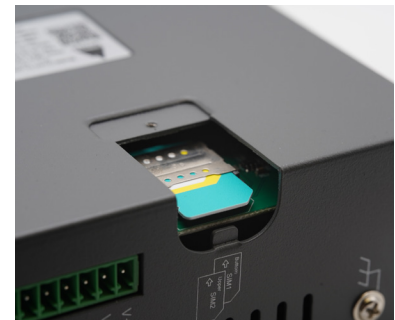
Figure 21. With one SIM fitted
