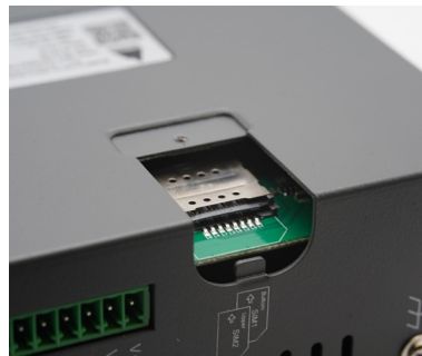
Figure 20. Dual SIM card holder
