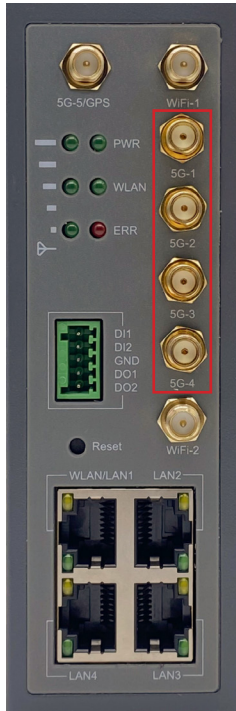
Figure 22. Cellular Antenna Connectors (GPS Version)
