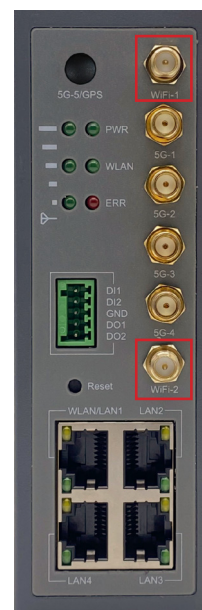
Figure 26. WiFi Antenna Connectors (non-GPS version)
