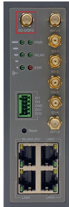
Figure 24. GPS Antenna Connectors (GPS Version)
